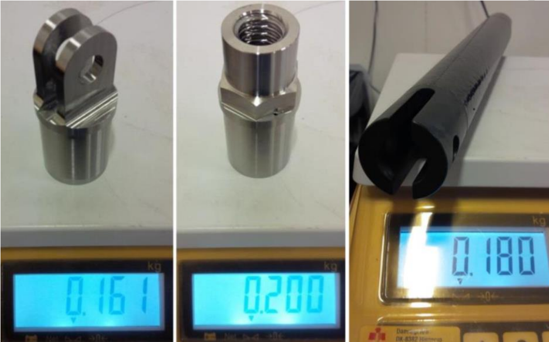
Figure 11 The whole strut has a mass of one equivalent INVAR metallic fitting
