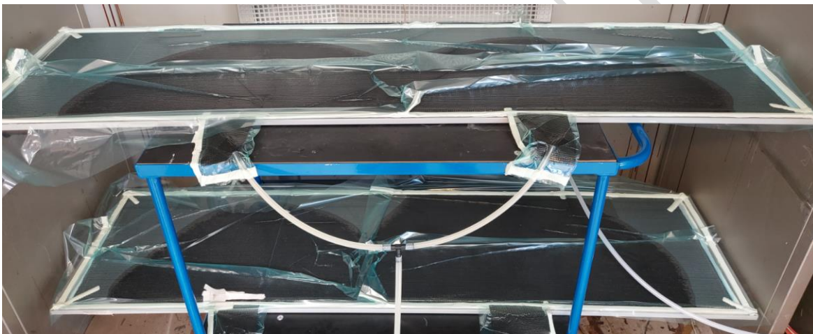
Figure 17 Thin flat CFRP panels vacuum infusion
