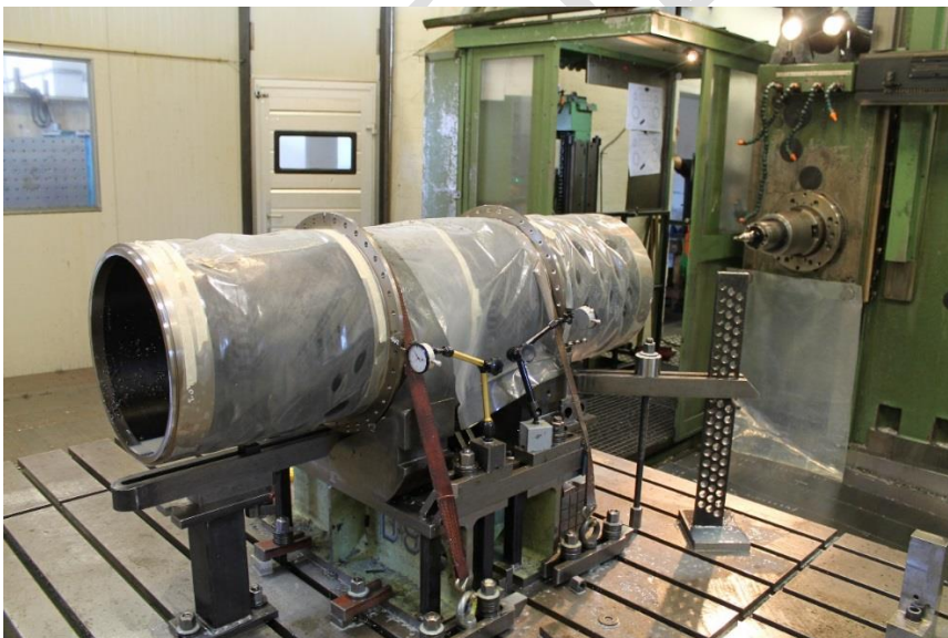
Figure 14 After-machining of bonded structure to achieve tight tolerances
