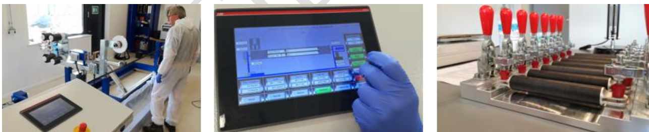
Figure 15 Inhouse manufacturing from left: Filament winding of CFRP tube, digital controlled CNC, struts in bonding jig
