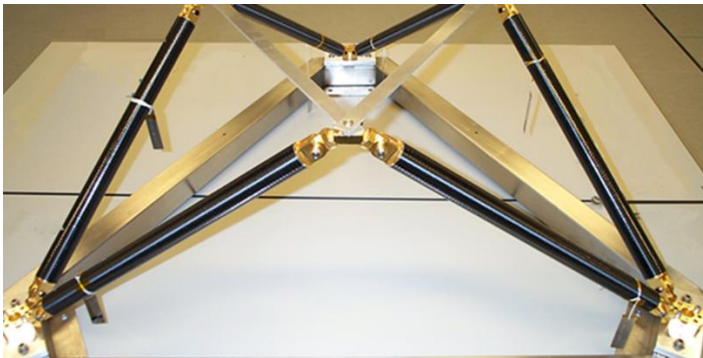
Hexapod struts shipped in formation
