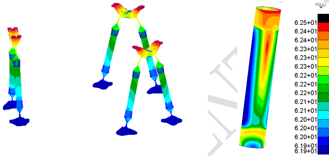
Figure 7 Deformation of the first axial mode + Thermal load on CFR Tube, cold
