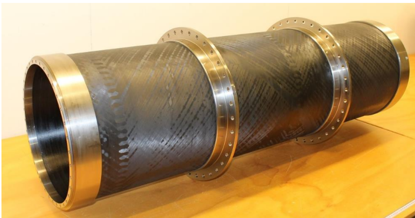
Figure 13 BASELINE: Monolith filament wound cylinder, example of Central tube similar size item
