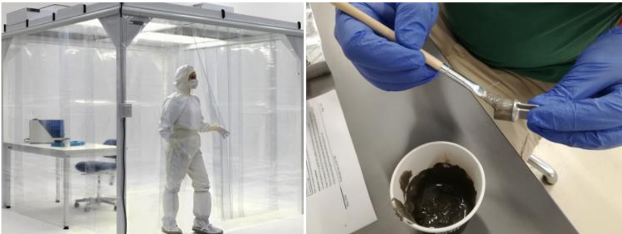
Figure 16 ISO 8 soft wall cleanroom (installed in October 2018), mainly for bonding, cleaning & contamination control purposes
