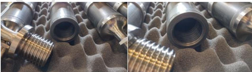
Figure 10 BLACK STRUTS, size Ø47, threaded fitting in action for ARIEL mission
